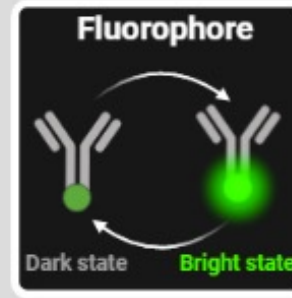
Laser pushes most fluorophores into a dark state
