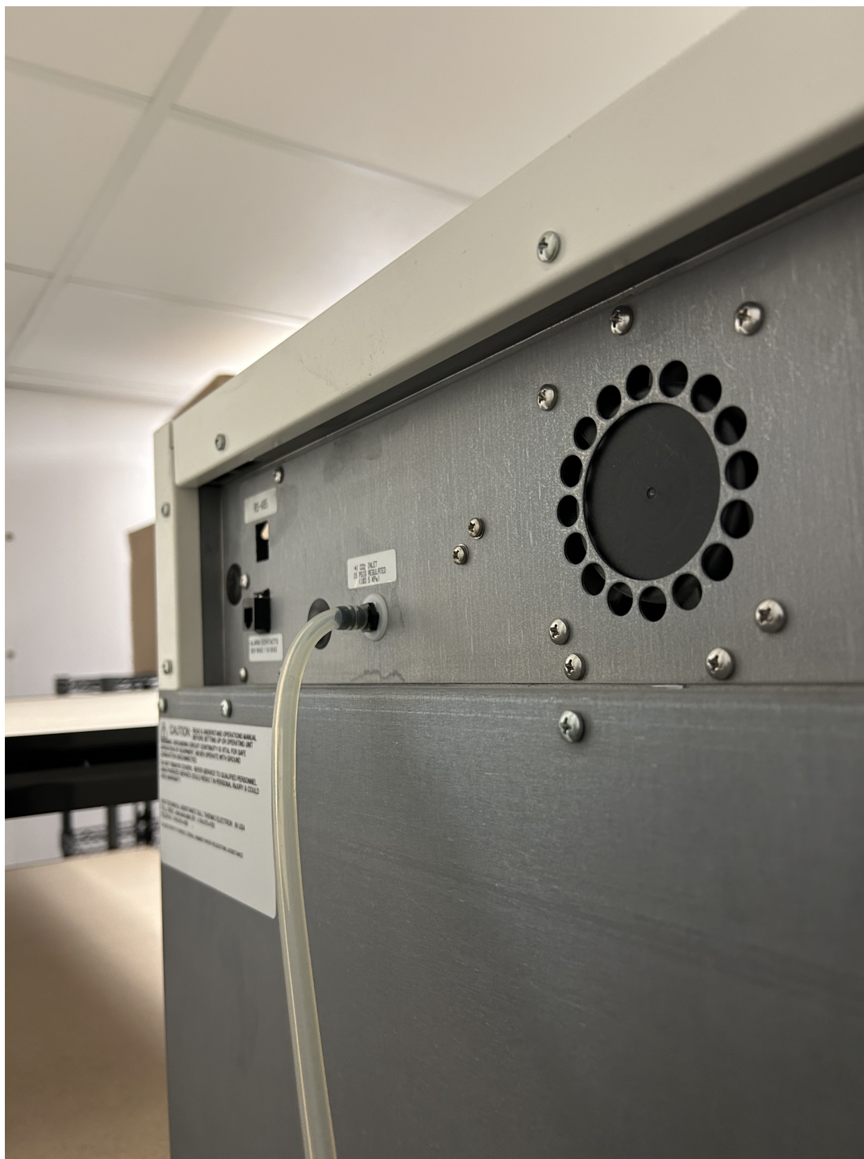
Fig. 6: Carbon dioxide tubing connected to the back of Maui (top incubator).
