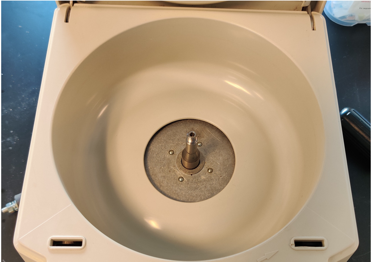
Fig. 1: The top of the microcentrifuge with the rotor removed.
