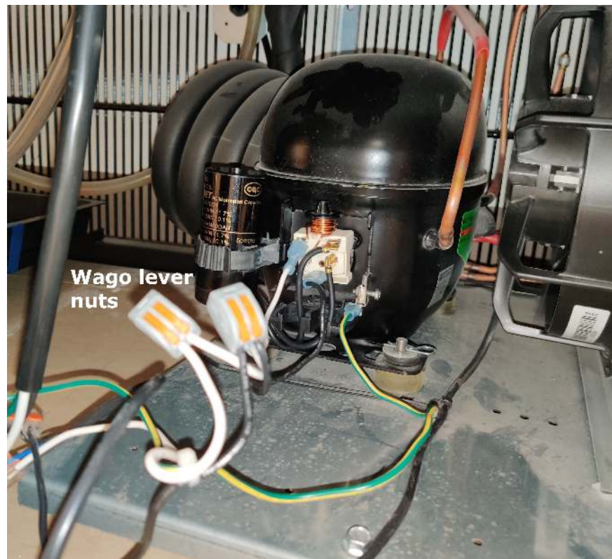
Fig. 14: The lever nuts are in the foreground, in their engaged position. You only need to lift the lever on the one wire we are removing for each lever nut.
