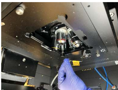
Fig. 13: Using labeled Allen wrench to tighten plate holder
