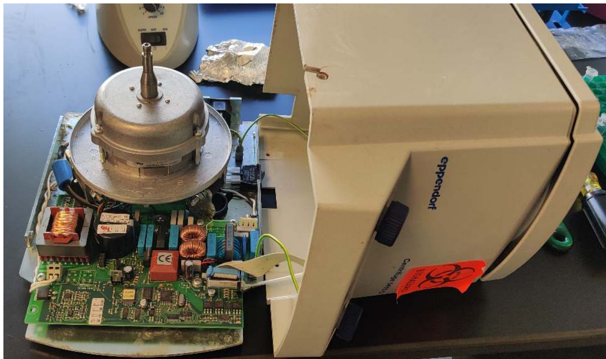
Fig. 2: The centrifuge with the shell removed. You should not disconnect the wires; just leave the shell on the right.
