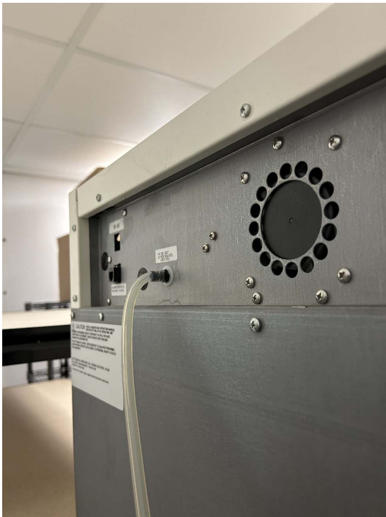
Fig. 7: Carbon dioxide tubing connected to the back of Maui (top incubator).
