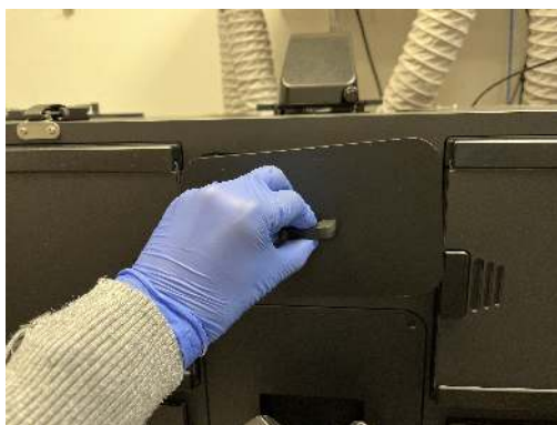
Fig. 7: Removing front magnetic window cover
