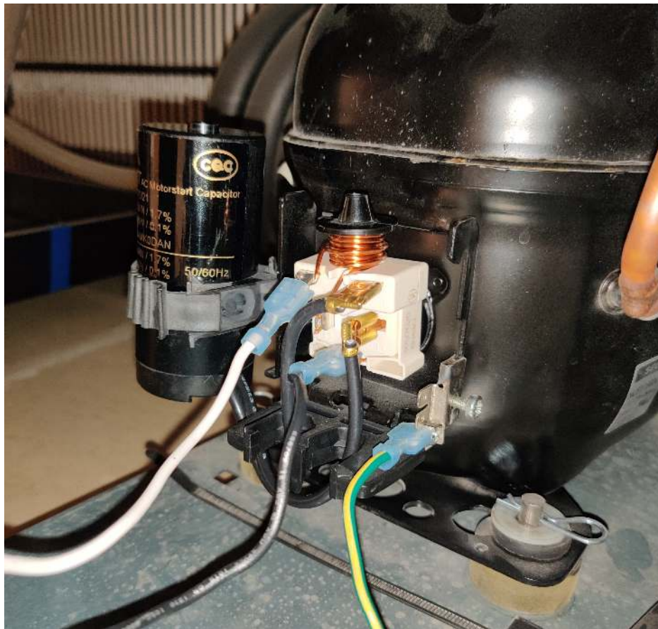
Fig. 17: Properly reassembled starter components
