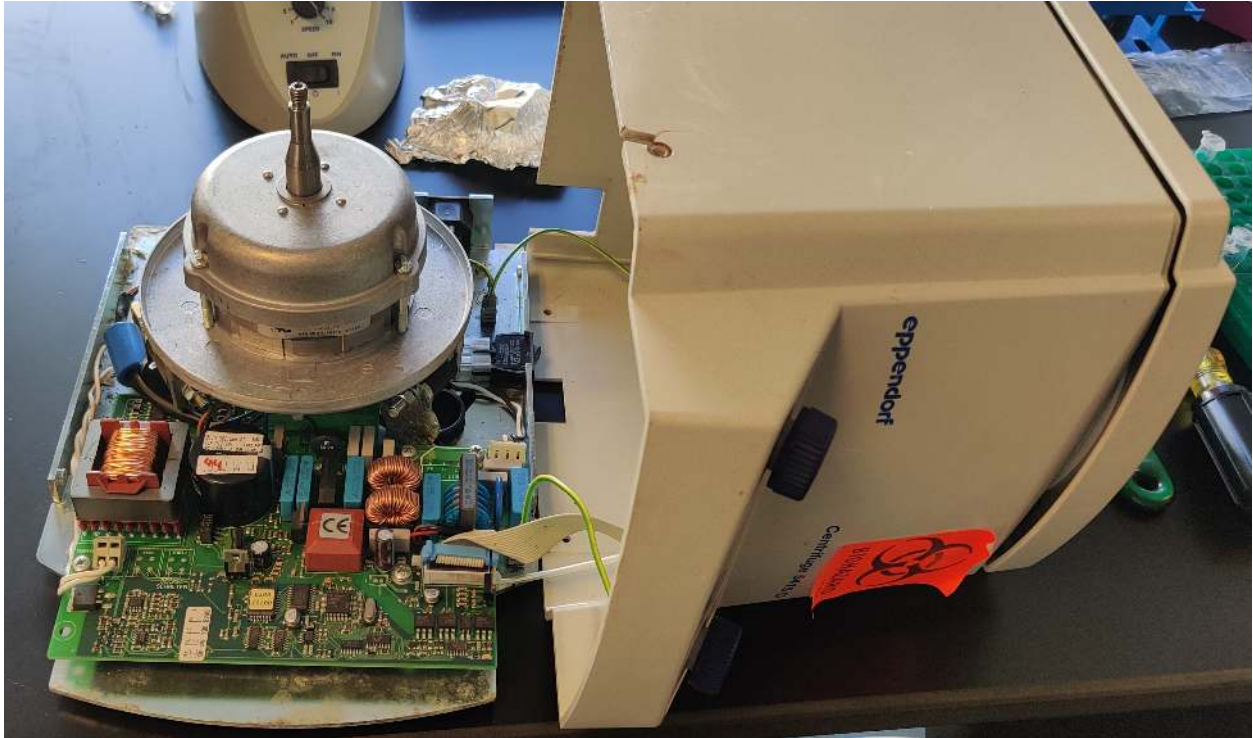
Fig. 2: The centrifuge with the shell removed. You should not disconnect the wires; just leave the shell on the right.
