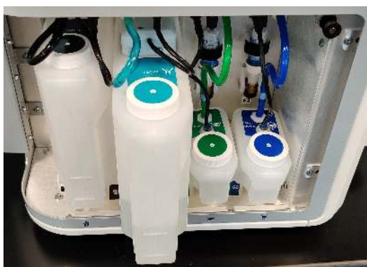
Fig. 2: The focusing fluid bottle can be moved slightly out for refilling without stressing the fluid or data line.
