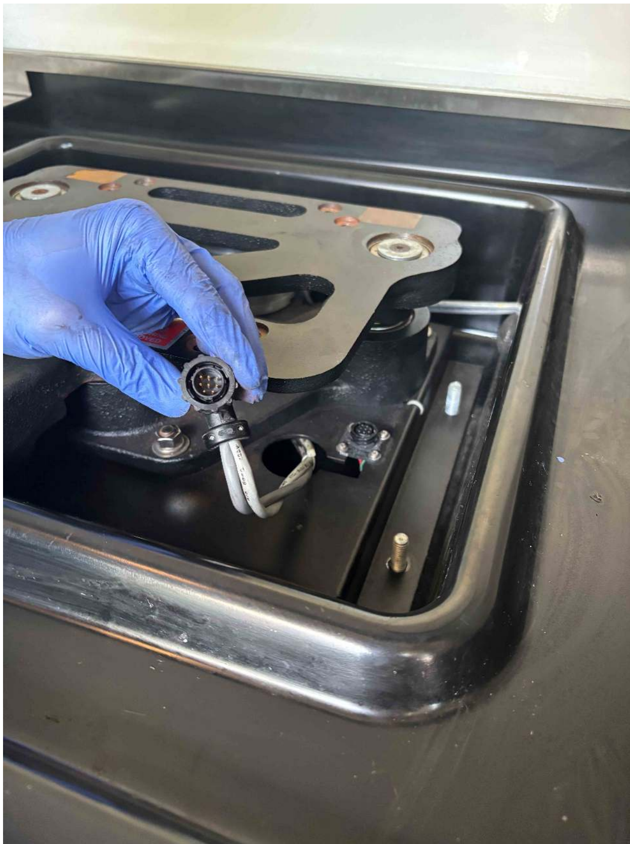
Fig. 23: Note the 3-3-2-pronged orientation that must match when being plugged in.
