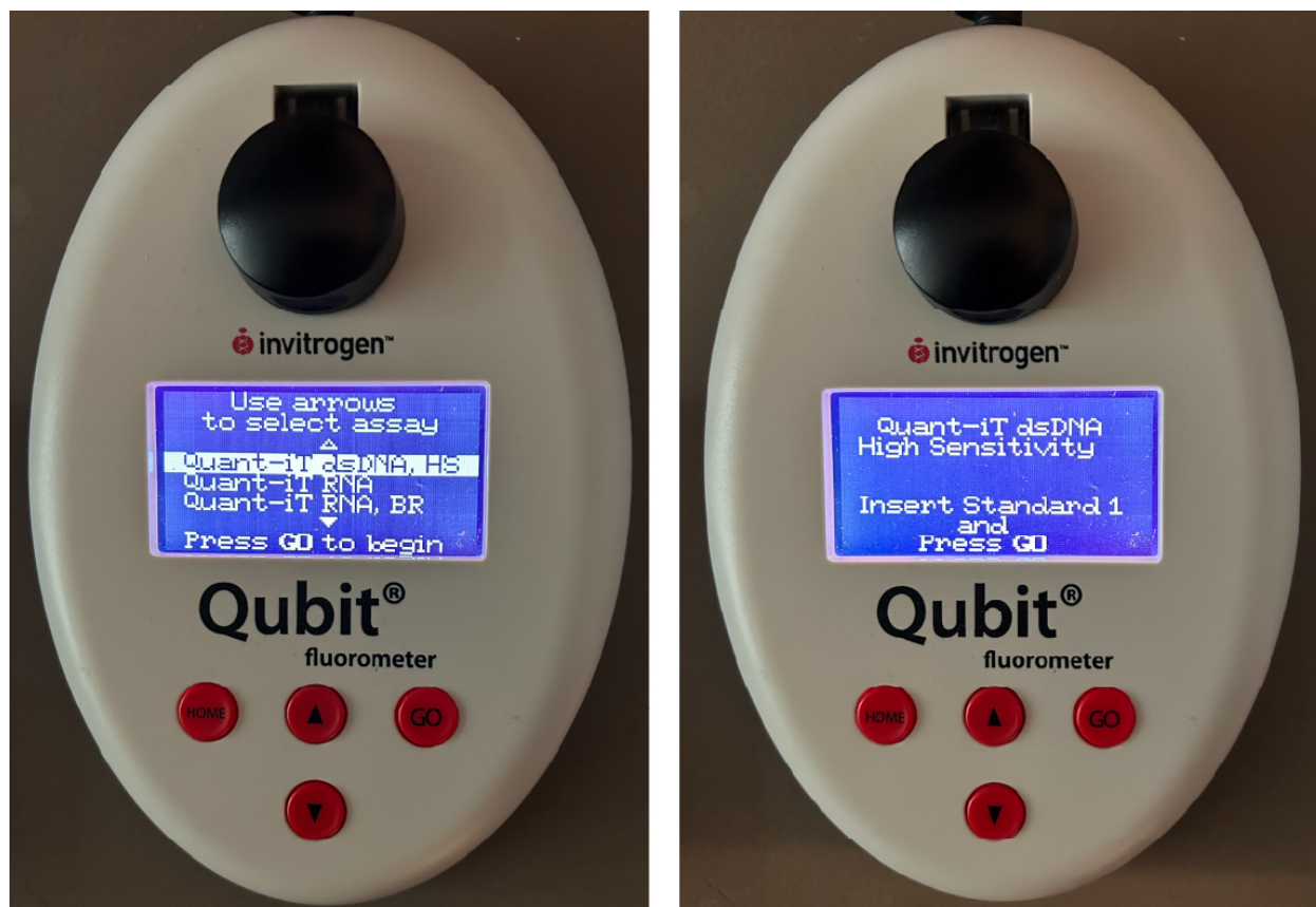
Fig. 21: Left: Choose the “dsDNA, HS” assay. Right: The instrument first prompts you to insert and measure Standard 1.
