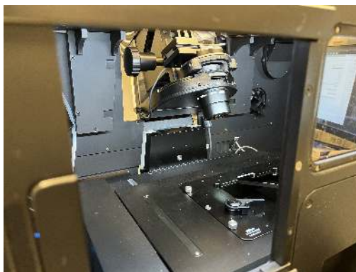
Fig. 12: Microscope pillar in “up” position relative to stage
